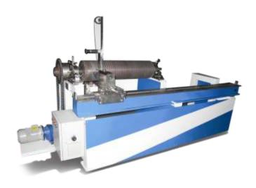
The All Roller Mounting Machine - ARM 08, is the result of years of experience in manufacturing and mounting of card clothing. With state-of-the-art features and user friendly design, ARM 08 makes perfect mounting of wires easy and effortless.
