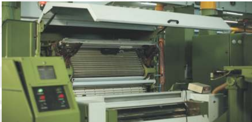
Tops Height Measurement & Resharpener on the Carding Machine
