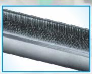
The effective removal of neps, short fibres and trash without rupturing fibres at high production rate requires unique positioning of wire points of the tops.
